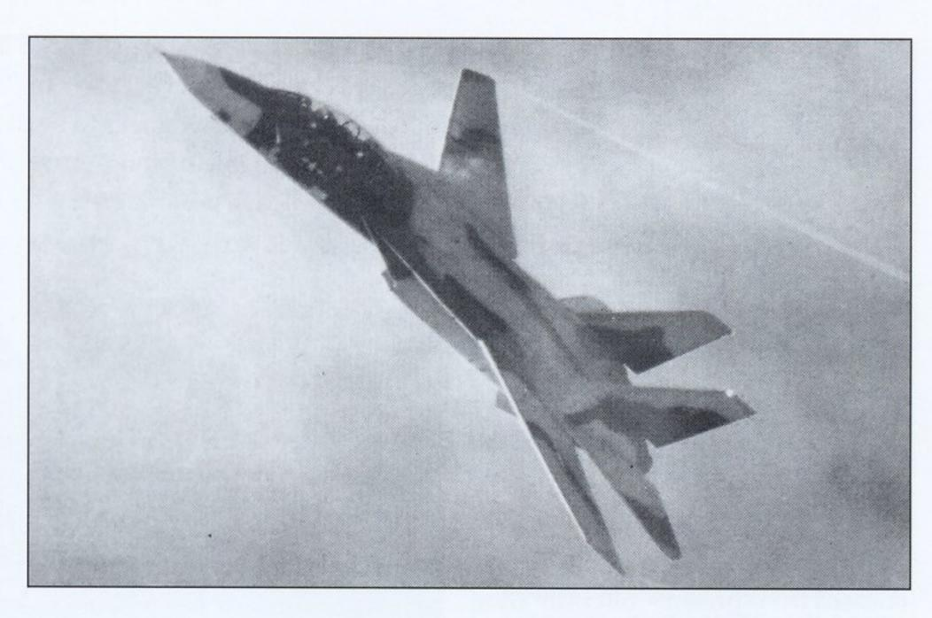
H-56 (BuNo 160354) breaks into the pattern overhead TFB 1 on finals. Note the vortices developing along the leading edge of the wings as the aircraft turns tightly in the moist air. Also of interest is the camouflage pattern on the uppersurfaces of the aircraft, the details of which are not often shown (authors' collection)
